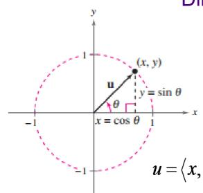
If  $\mathbf{u}$  is a unit vector such that  $\theta$  is the angle (measured counter clockwise) from the positive x-axis to u, then the terminal point of  $\mathbf{u}$  lies on the unit circle
